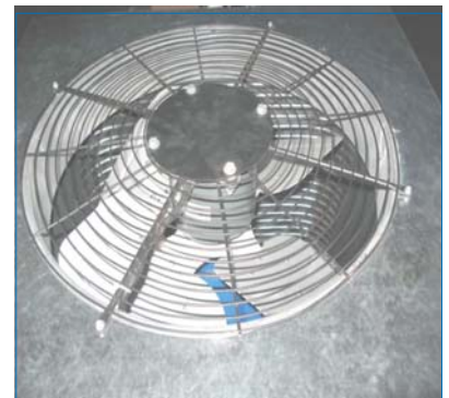
Figure 1 : Condenser Fan Motor arrangement for Models APMR 61060-62180
